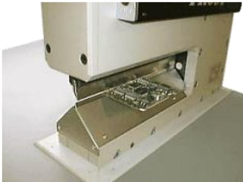
In order to automatically assemble printed circuit boards in an economical way, the multiple printed circuit board technology is used nowadays. Delimitation of the single printed circuit board is achieved by mill-cutting, perforation or carving. The development tends more and more towards the technique of carving; it means low costs and a high degree of stability and has favourable effects on assembly and soldering. Conventional separation
